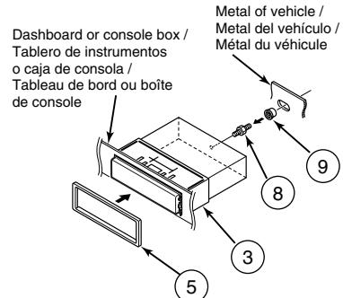
**If installing the main unit using the side brackets of the vehicle**
