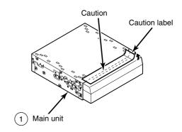
Mounting the main unit (If installing the main unit using the mounting sleeve)
