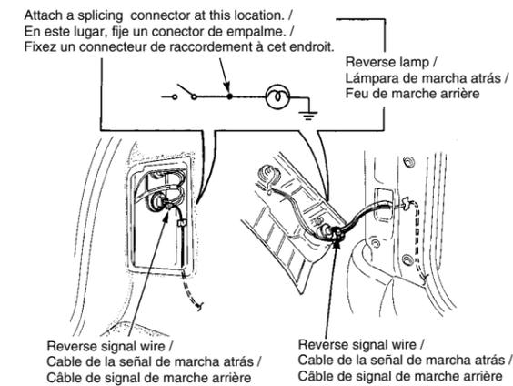
Using the splicing connector
