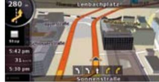
The lane that should run is displayed on the screen by a guiding arrow when there are two or more lanes. By following the arrow you cannot miss turning in the divergence point so that you can drive smoothly even in difficult situations.
