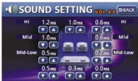
Complex to perform manually, optimal delay settings can be adjusted automatically for the various speakers in the system for true time alignment. For experienced users, more tweaking is possible in the manual mode.
