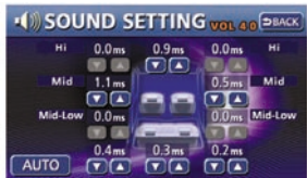
Fullrange speakers can be time-aligned automatically with the AUTO setting. One single push is all that's needed for the whole process.
