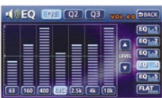
Simpler parametric equalisation function can adjust the "Q," i.e. bandwidth, of each of the 7 centre frequencies from wide to narrow in 3 steps.
