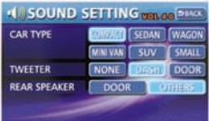
A simpler time alignment performed by selecting the car type and speaker positions, then adjusting each speaker level. Delay parameters are then adjusted for a time-aligned response.
