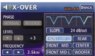
Adjusting a crossover point's frequency, rolloff using "slopes" from bandpass to 6/12/18/24dB/octave and level settings.
