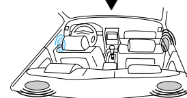
"Turn" Audio muted Music cuts off at the front left speaker and the navigation voice message is heard.
