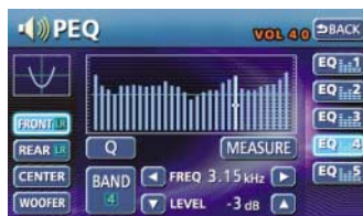
To suit preferences and music genres, up to five sets of user-configured PEQ settings can be preset and stored in memory for instant recall.
