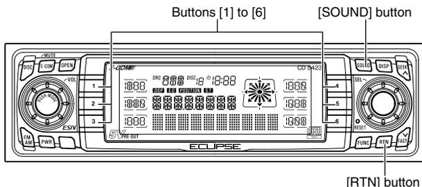
**4 Hold down a button, [1] to [6], for more than two seconds to preset a value.**
