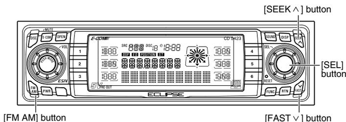
First, press the [FM AM] button to start tuner operation.
