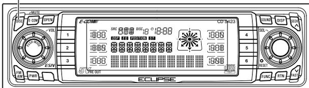
First press the [DISC] button to switch to the disc mode. It is assumed here that a CD has already been loaded into the unit.
