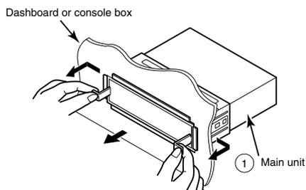
–Mounting the main unit (If installing the main unit using the side brackets of the vehicle)–
