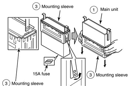
– Mounting the main unit (If installing the main unit using the mounting sleeve) –
