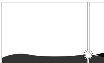
\*Smear effect: A phenomenon where a vertical line appears from a high-luminance point striking the camera (such as the reflection of the sun's rays on the chassis).
