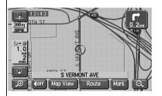
Signals are received from 3 or more GPS satellites to pinpoint the present location of your vehicle. The device will display a **GPS** mark on the upper left part of the present location screen when it is receiving signals from 3 or more satellites and positioning is rendered possible.
