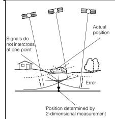
The GPS calculates your position using a 3-point measurement principle.
