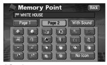
• Selecting a symbol with sound will enable an alarm to sound when about 0.3 miles from the memory point.
