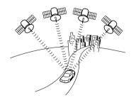
The GPS is a system that uses signals received from a satellite in a maximum orbit of approximately 21,000 km above the earth to indicate your present position (latitude, longitude, altitude).
