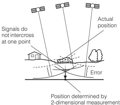
GPS calculates the position using the triangulation.
