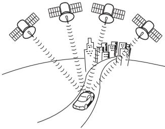
GPS is a system to detect current location (latitude, longitude, altitude) by receiving radiowaves from normally 4 or more, or 3 in some cases, GPS satellites orbiting 21,000 km over the Earth.
